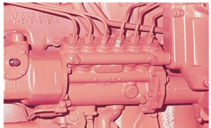
Figure 1-6. Diesel injection pumps are quite complex and must be built to exacting tolerances. (Caterpillar)
