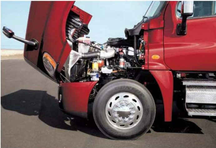
Figure 2-6. When working on an engine, be sure that the hood is in the locked position and is well supported. (Daimler AG)
