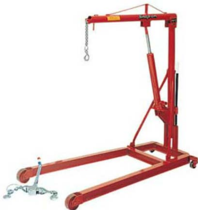
Figure 2-7. When removing an engine, use a lift that is rated to do the job. This lift is sometimes referred to as a "cherry picker." (Snap-On Tools)
