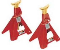
Figure 2-5. Jack stands should be used whenever you must work under a vehicle. Be sure to locate them under the vehicle's frame, not under a drivetrain or suspension part. (Snap-On Tools)
